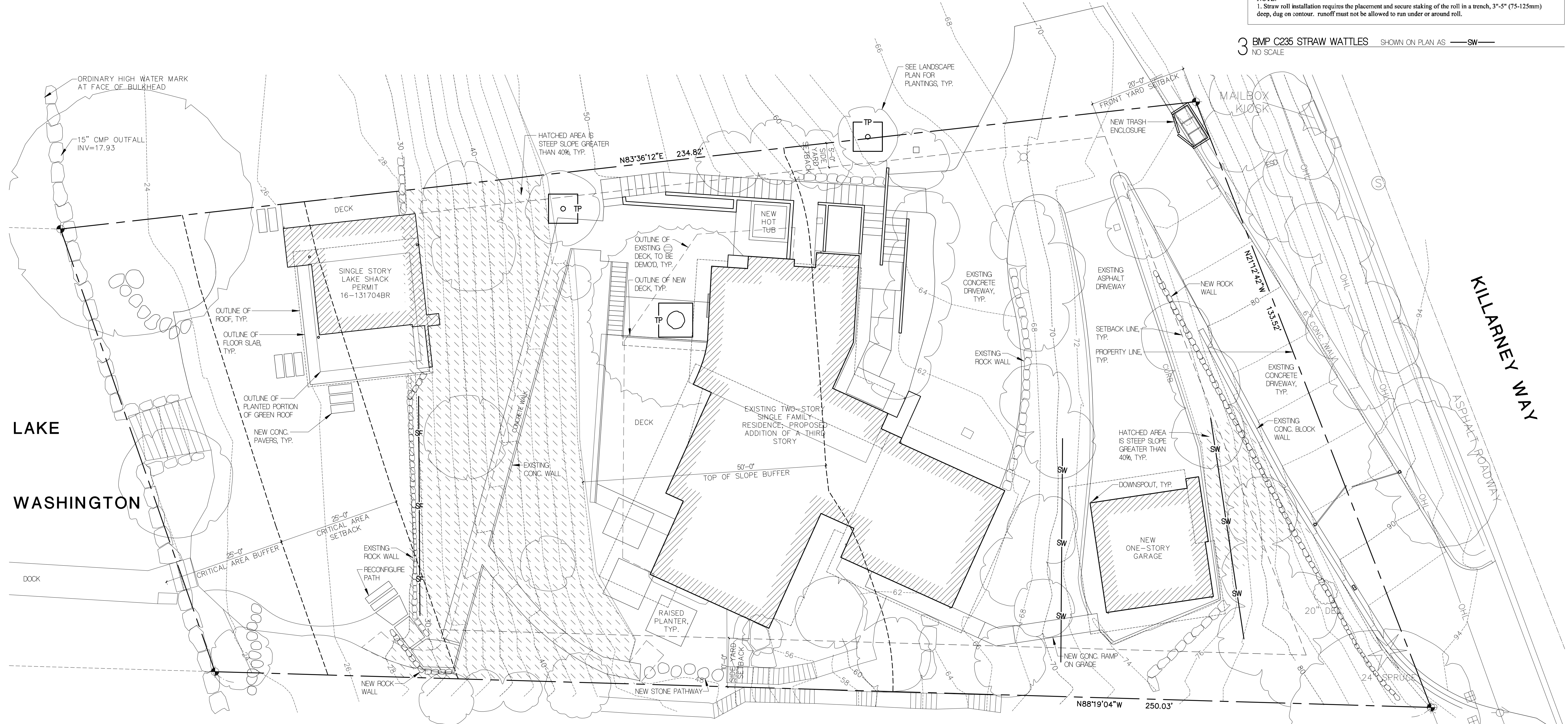
1 CONSTRUCTION STORMWATER CONTROL PLAN T = 10'-0"
